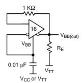
Figure 22. V<sub>BB</sub> Voltage Reference Generator
