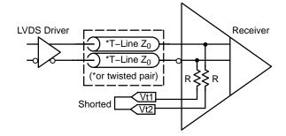
**Internal Termination Singulated Pins**
