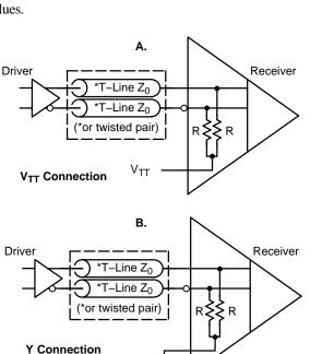
$V_{EE}$ Figure 5. Combo Pin V<sub>TT</sub> or "Y" Connection with **Internal Parallel Termination**
