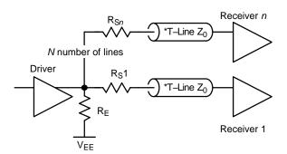
Figure 17. Parallel Fanout Using Series Termination
