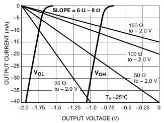
Figure 11. Normal Output Levels Driving Various Load Impedances
