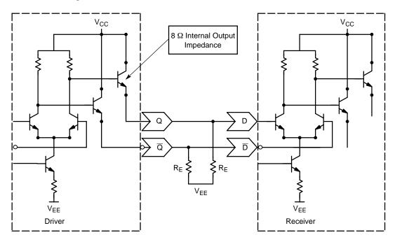
Figure 1. Typical ECL Output with Emitter Follower Output Structure, Typical Termination, and Typical ECL Input Interconnect
