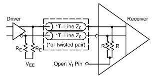
Internal Termination Combo Pin Figure 8. Standard Pair Termination with Internal Termination
