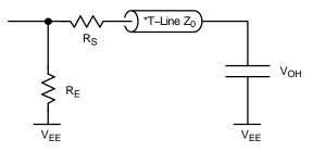
Figure 16. Equivalent Circuit with Output Cutoff
