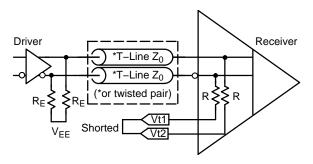
**Internal Termination Singulated Pins**
