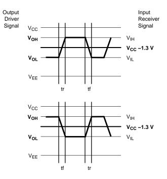
Figure 2. State Levels V<sub>OH</sub>, V<sub>OL</sub>, and Dynamic Transitions at Q or  $\overline{Q}$  and D or  $\overline{D}$
